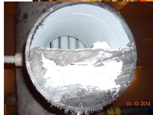
Removal of sodium-contaminated piping
