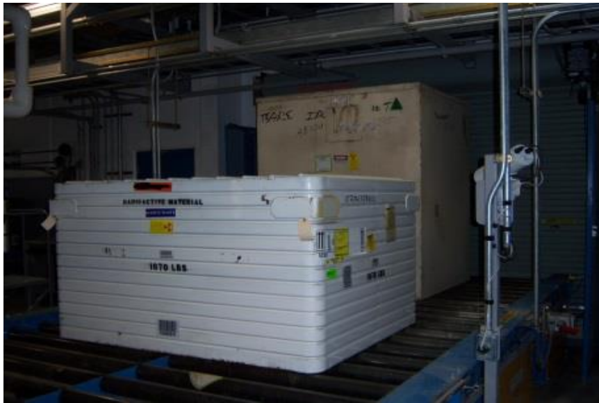
LANL Corrugated Metal Box on conveyor for Boxline processing
